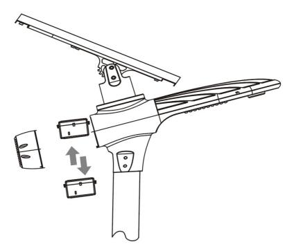
Battery replacement just need opening rear cover and replace with new battery directly, no need of taking apart whole luminary.
