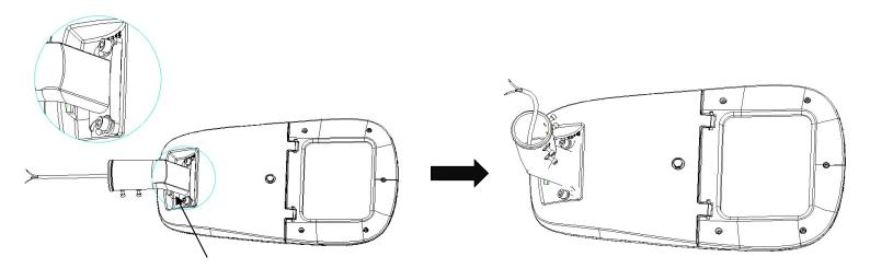
1. 2 Wire the fixture according to L(Brown), N (Blue), PE(Green-Yellow), and top mount the fixture on to a straight pole. Adjust the fixture in an angle which you want, Then fasten the screws. Add the photocell sensor if you have.
