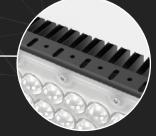
The module heat sink adopts the hemming design to prevent the deformation of the heat sink due to crash during the shipment and enhance the flatness and strength of the contact surface of the module heat sink.
